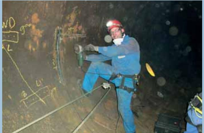
Tests on the welding seams of the penstock pipelines
