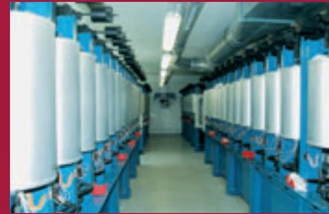
View of a creep rupture test lab with single oven units
