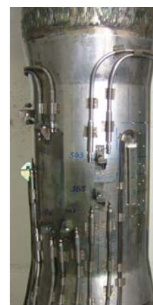
Fig.6-Sensor application on test pipe P22-P91
